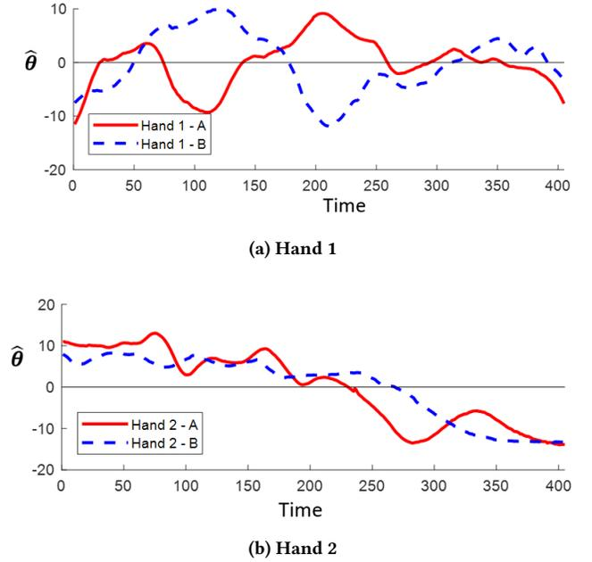
**Figure 5: Comparison of the verticality angle  $\hat{\theta}$  (in degrees) for the Hand datasets with Subject A (red, solid) pulling and Subject B (blue, dotted) being pulled.**
