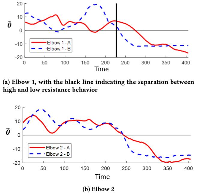
**Figure 6: Comparison of the verticality angle  $\hat{\theta}$  (in degrees) for the Elbow datasets with Subject A (red, solid) pulling and Subject B (blue, dotted) being pulled.**
