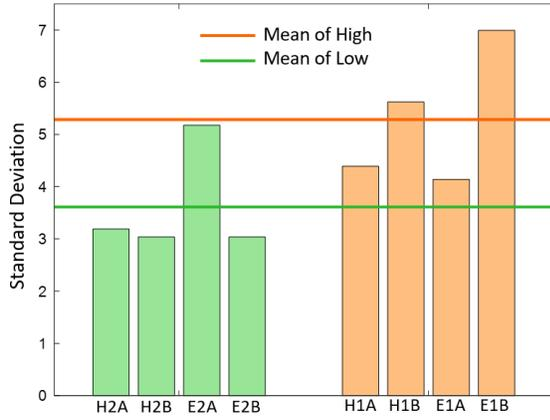
**Figure 9: Comparison of the standard deviation of the difference of each signal from its linear resistance, separated by higher (green) and lower resistance (orange). Also pictured is the mean of the each subgroup, which shows the higher mean of the higher resistance group. The labels along the x-axis correspond to hand or elbow (H/E), video number (1/2), and subject (A/B).**
