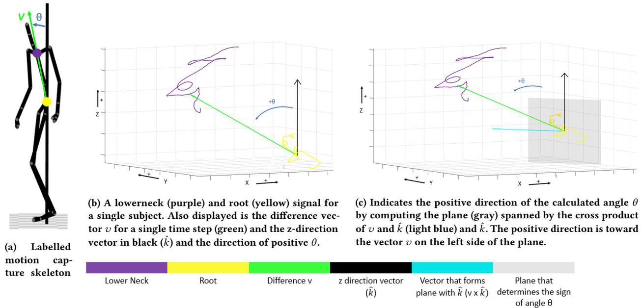
Figure 3: Process from the motion capture data to the angle between the difference vector  $v$  and the vertical direction  $\hat{k}$
